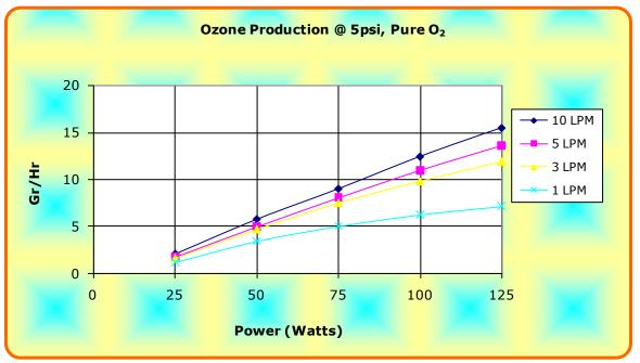
Normal factory POWER set point: 125 watts at FULL PDM (10vdc or 20ma).
