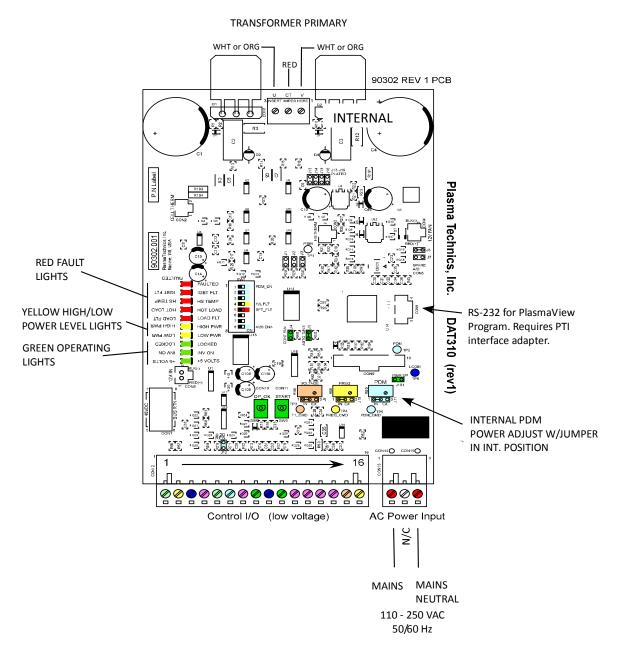
115 VAC wiring should be rated 10 Amps.
