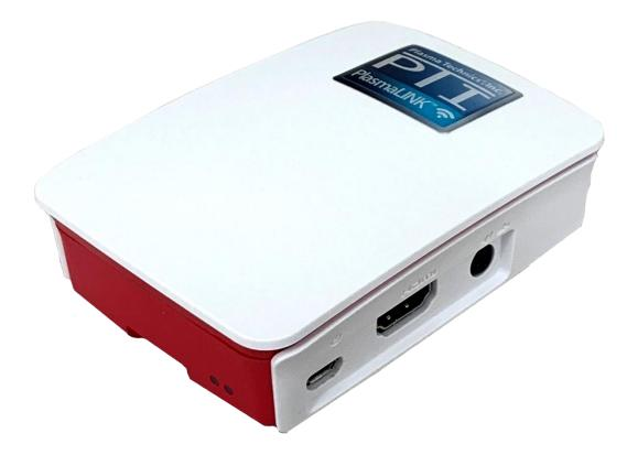
A **new** way to connect and communicate with your **Plasma Block**<sup>®</sup>. The PlasmaLINK unit connects to the DAT series board on Plasma Block<sup>®</sup> units.
